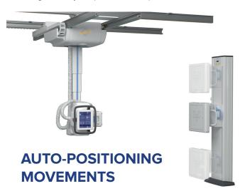
The ceiling suspension automatically moves to the center of the detector, located in the table or the wall-stand, according to the SID and angulation of the tube. All axes are servo-assisted and motorized for travelling up to 16.4 feet and 360° angles.
