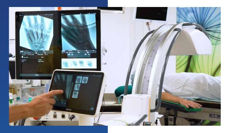
Perfectly balanced orbital and angular rotation of the C-arm for fast and precise positioning. Responds perfectly to operator touch and feel.
